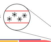
Custom hollow core fibre for mode-matching with single mode fibre.
